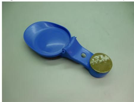
6. Inspect the tab opening of the pan. Inside opening should be between 48mm to 52mm. If not, adjust tabs by bending tabs.
