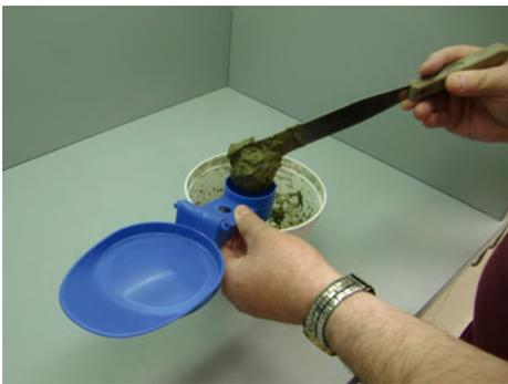
5. Let the mixture dry sufficiently. The dried counterweight should weigh around 140g.
